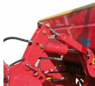
A-frame mounting for pneumatic seed drills.
