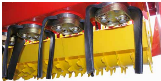
The pin and lynch pin are well protected from dirt.
