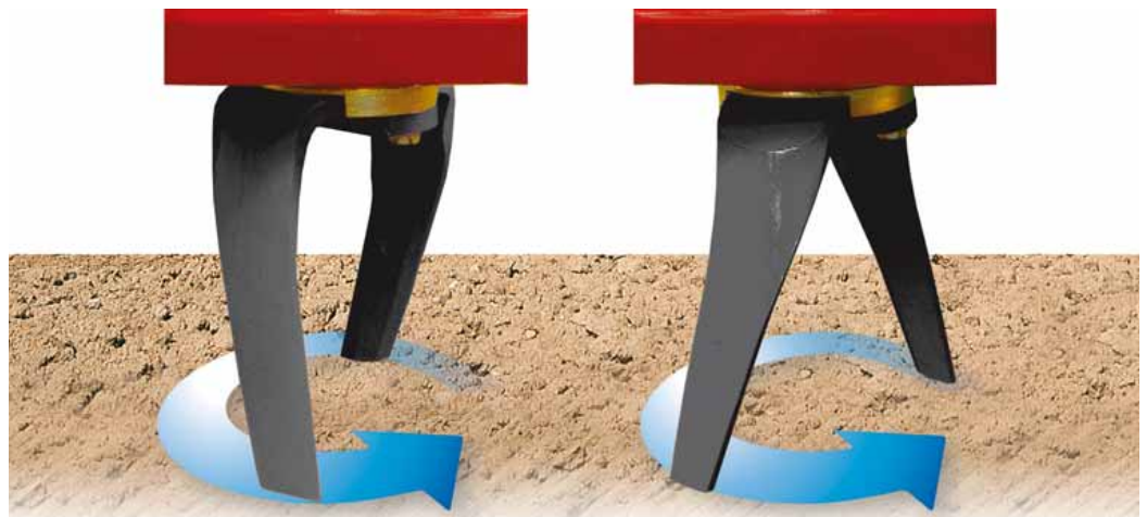
Tines in aggressive position – the ground is broken up
