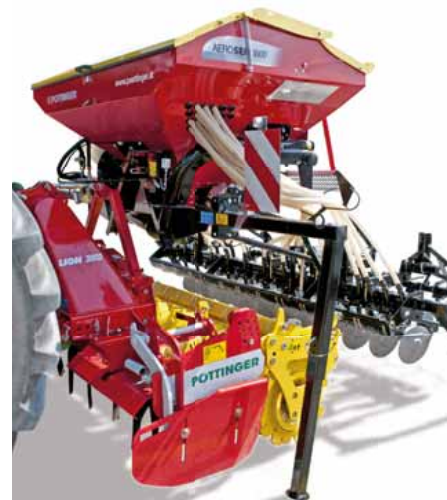
A-frame mounting for pneumatic seed drills.
